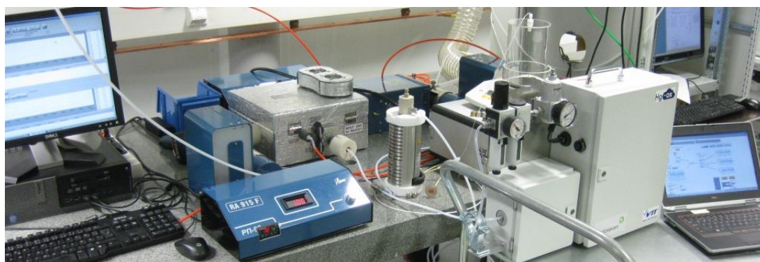
Figure 1. The dual analytical system by Lumex Analytics GmbH in operation with gas generators.
