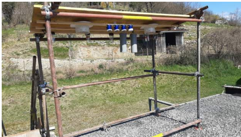
Figure 14. Installation of passive samplers at Vodarna site.
